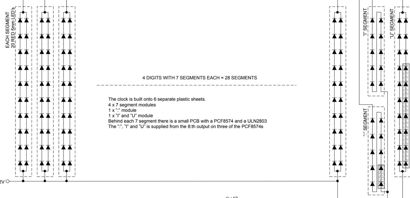
The clock is built onto 6 separate plastic sheets.
